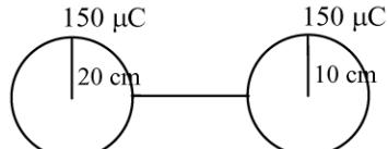
$$\begin{aligned} V &= \frac{Q_1 + Q_2}{C_1 + C_2} = \frac{150 \times 2 \times 10^{-6}}{4\pi\epsilon_0(r_1 + r_2)} \\ &= \frac{300 \times 10^{-6} \times 9 \times 10^9}{30 \times 10^{-2}} \\ &= 9 \times 10^6 \text{ V} \end{aligned}$$
